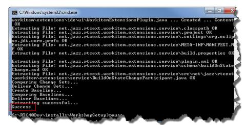
In case of errors, carefully read the error message, check the paths, especially to your Java JDK and make sure it is available.
