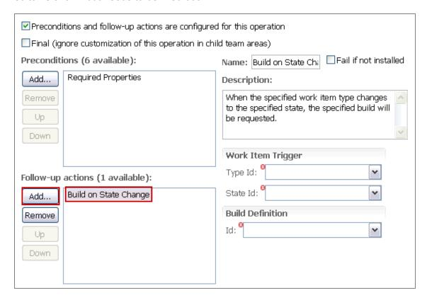
\_\_d. Fill in the **Work Item Trigger** as shown here. You may, of course, choose different values for the work item type and state, but then you will need to adjust the following steps accordingly.
