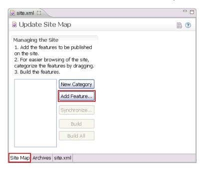
\_\_d. In the **Feature Selection** dialog, type \*rtcext into the filter, select the feature you created in the last section and then click **OK**. Back on the site.xml editor type **Ctrl+S** to save the file.
