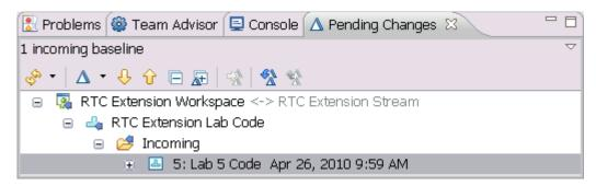
\_b. Right click the Lab 5 Code change set under the RTC Extension Workspace node, and then click the Expand Children action. This will reveal all the changes made for lab 5. As you can see the full change is the addition of a new plug-in project. The first entry shows a folder addition to the root. That folder contains all the other additions in the following changes. You will next load the code and then go through it in detail.
