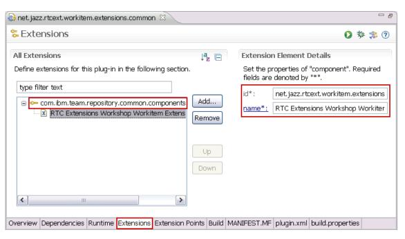
\_\_d. Back in the **Package Explorer** view, expand the src/net.jazz.rtcext.workitem.extensions.common source package and then double click the **IComponentDefinitions.java** file. This file contains constants that pertain to the component as a whole. In this case there is just a constant for the component's id.
