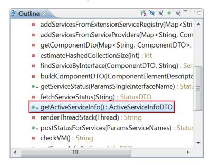
\_\_f. The editor is now showing the **getActiveServiceInfo()** method. Set a breakpoint on the first line of the method. Right click in the shaded area to the left of the first line to get the menu.
